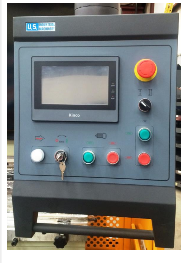
Photo above is "Simple CNC". This control is CODE ONLY, with touch screen input. This allows 2-axis programming of X (backgauge) and Y1 (ram position).
