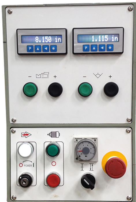
Photos above are MANUAL Hydraulic Press Brake with front-operated power backgauge, power ram adjustment, both with manual fine adjustment and digital readouts. Operators pendant has dwell adjustment for ram, key lockout, jog control and E-stop.
