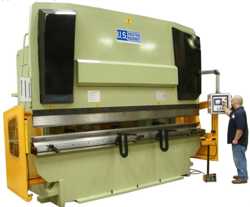
Photo above shows a 330 ton x 13' press brake with CNC.
