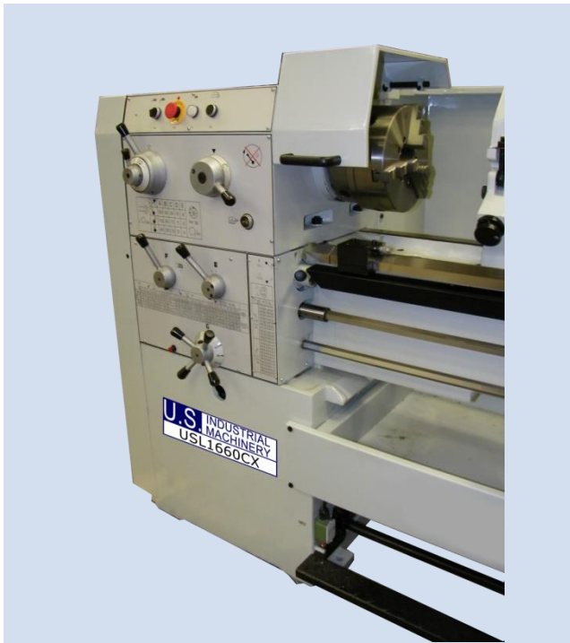
Detail of Headstock, chuck and guard
