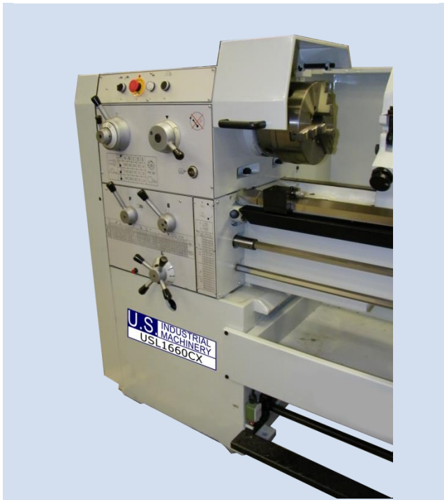
Detail of Headstock, chuck and guard
