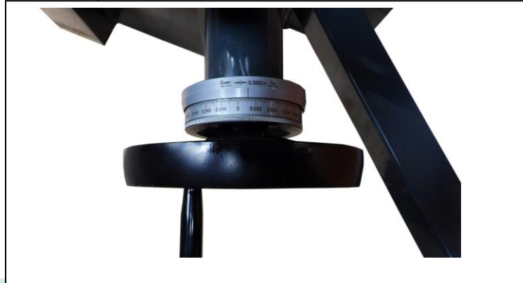
Detail of manual fine adjustment of downfeed with 0.0002" graduations
