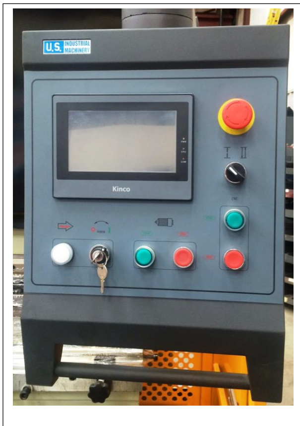
Photo above is "Simple CNC". This control is CODE ONLY, with touch screen input. This allows 2-axis programming of X axis (backgauge) and Y1 (ram position).
