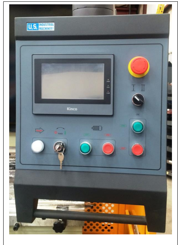
Photo above is "Simple CNC". This control is CODE ONLY, with touch screen input. This allows 2-axis programming of X axis (backgauge) and Y1 (ram position).
