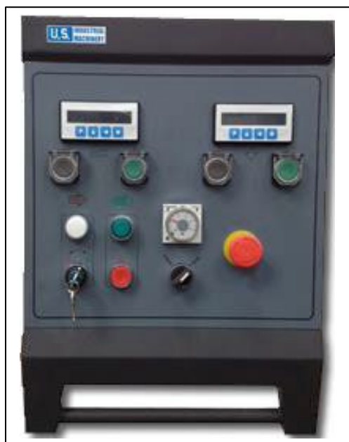
Photos above are manual Hydraulic Press Brake with front-operated power backgauge, power ram adjustment, both with manual fine adjustment and digital readouts. Operator's pendant has dwell adjustment for ram, key lockout, jog control and E-stop.
