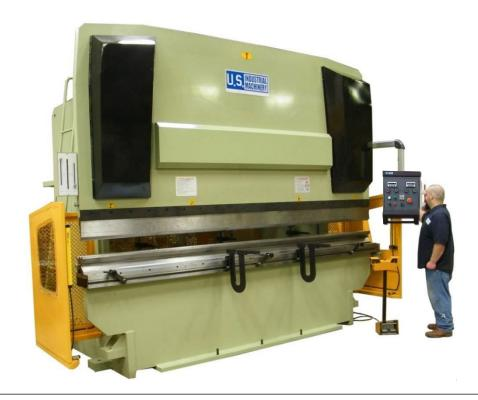
The manual machine will have the control pendant shown on the left. Front operated power backgage, power ram adjustment, both with manual fine adjustment and digital readouts. Operator's pendant has dwell adjustment for ram, key lockout, jog control and E-stop.
