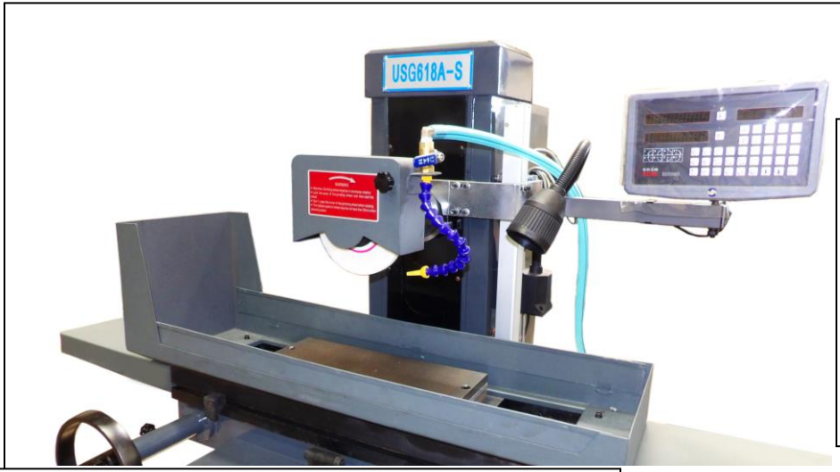
Detail showing permanent magnetic chuck, 2-axis digital readout display, flood coolant nozzle, worklight.
