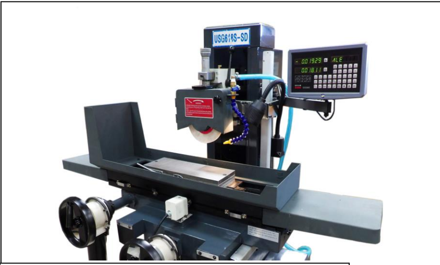
Detail showing permanent magnetic chuck, over wheel diamond dresser, 2-axis digital readout display, flood coolant nozzle
