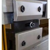
Our **optional** ram clamps for all punch Tangs shown above. Lever action allows for quick tool change.
