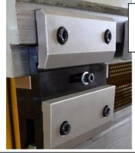
Our **optional** ram clamps for all punch Tangs shown above. Lever action allows for quick tool change.
