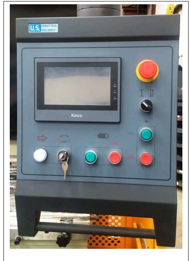
Photo above is "Simple CNC". This control is CODE ONLY, with touch screen input. This allows 2-axis programming of X axis (backgauge) and Y1 (ram position).
