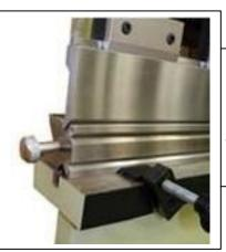
Gooseneck Punch Tool Sections included, full length of Ram. Multiopening V-Die for up to 90 degree forming included, full length of bed. Die lifting rings included.
