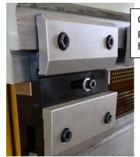
Our **standard** ram clamp for all punch tangs above, two allenhead cap screws to secure tools.
