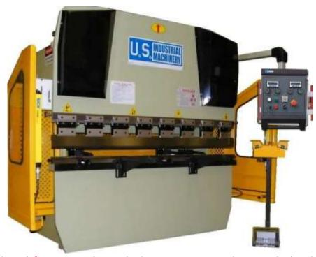
Photos above are manual Hydraulic Press Brake with front-operated power backgauge, power ram adjustment, both with manual fine adjustment and digital readouts. Operator's pendant has dwell adjustment for ram, key lockout, jog control and E-stop.
