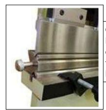
Gooseneck Punch Tool Sections included, full length of Ram. Multi-opening V-Die for up to 90 degree forming included, full length of bed. Die lifting rings included.
