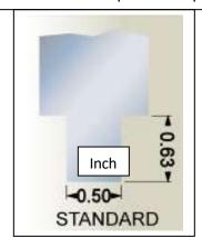
Our **standard** ram clamp for all punch tangs above, two allenhead cap screws to secure tools.
