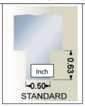
Our **standard** ram clamp for all punch tangs above, two allenhead cap screws to secure tools.
