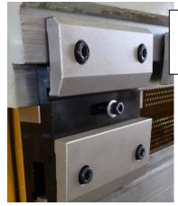
Our **optional** ram clamps for all punc Tangs shown above. Lever action allows for quick tool change.
