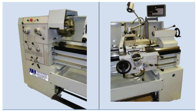
**QUICK CHANGE TOOLPOST OPTION – (Replaces standard four-way toolpost**
